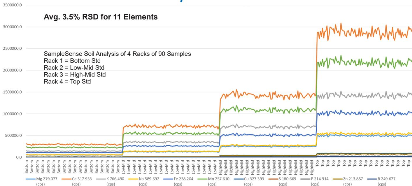
Analysis of 360 samples in 35 minutes. The four levels represent a rack of 90 samples, with each of the four calibration standards levels individually loaded with 5 mL of liquid into each of the 90 positions contained in each rack. Excellent stability observed from within each of the four concentration levels.
