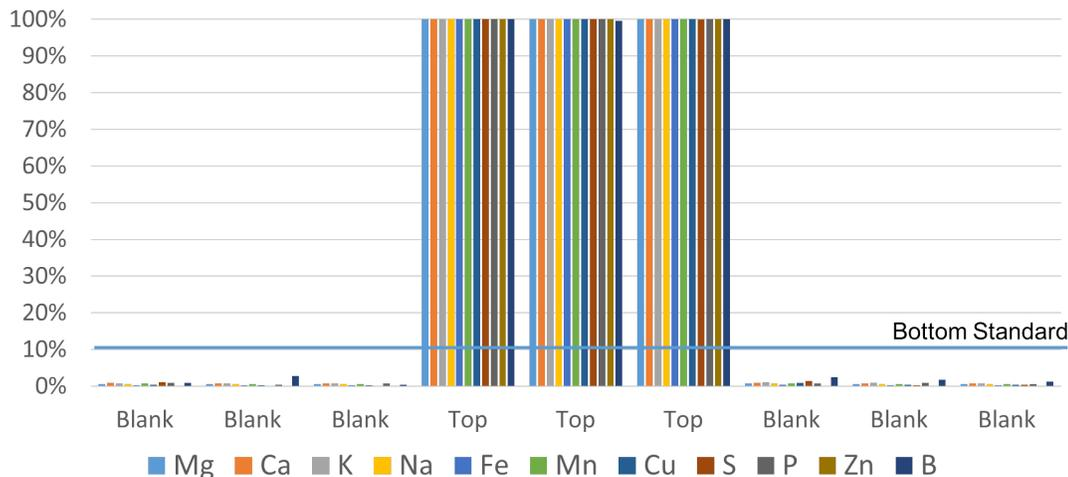
The SampleSense Soil rinse-out immediately reduces all elements to concentrations well below the bottom standard when using the six second Mehlich-3-ICP procedure. Additional seconds can be added to the rinse-out to meet lab requirements. The system can deliver rinse-out factors of 1,000x, 10,000x or more depending on how clear the spray chamber needs to be before the next sample is introduced.
